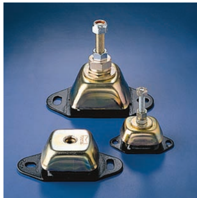
Mackay M2000, M2200 & M2400 Mounts (HVAC, Equipment, Engine & Cab) (Series 1: 50 – 100 kg @ 4 mm) (Series 2: 135 – 450 kg @ 5 mm) (Series 3: 355 – 1000 kg @ 5 mm)
