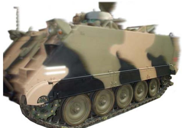
The excellent relationship between the DMO, DSTO and Mackay resulted in the production of a track shroud that was better designed and less expensive than the imported alternative, and 16% lighter in weight.
